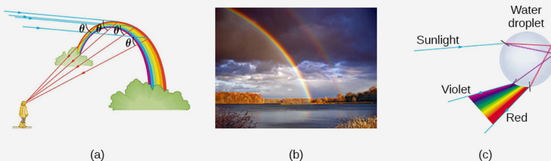
Figure 5.13 Rainbow Refraction. (a) This diagram shows how light from the Sun, which is located behind the observer, can be refracted by raindrops to produce (b) a rainbow. (c) Refraction separates white light into its component colors.
